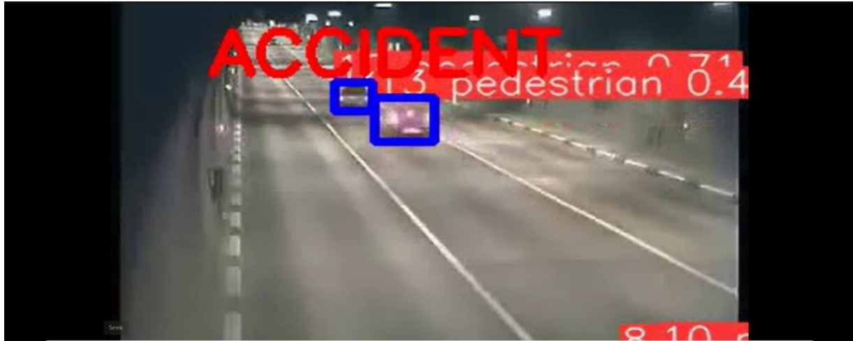
Figure 5: Shows the accident detection output where objects are highlighted with bounding boxes and an “ACCIDENT” alert is displayed for critical events.
